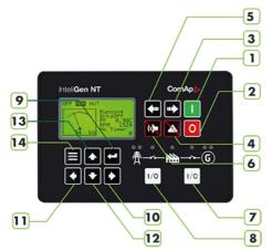
1.Start 2.Stop 3.Mode > OFF > MAN > AUT > TEST 4.Fault Reset 5.Mode < OFF < MAN < AUT < TEST 6.Horn Reset 7.GCB control (Open/Close) 8.MCB control (Open/Close) 9.Enter 10.5% Increase of edited setpoint's value. 11.5% decrease of edited setpoint's value. 12.Decrease setpoint value. 13.Increase setpoint value.
